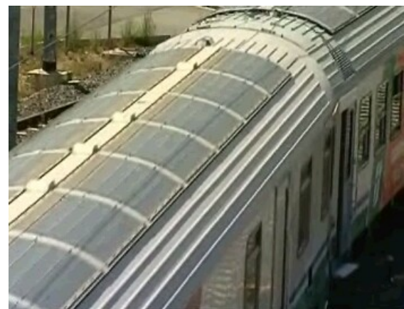
Image 5: Solar roofing on the conventional passenger cart.
